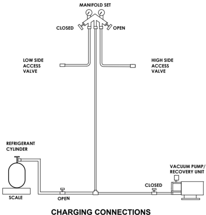
2. Close the vacuum pump valve, the low side service valve, and the low side manifold gauge valve.
