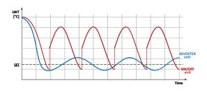
Normally, the capacity supplied by the unit exceeds the capacity actually required by the system.
