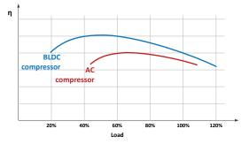
As can be seen in the diagram, a brushless motor is more efficient than a normal asynchronous motor and its efficiency reaches its maximum when the compressor is working under partial load conditions.
