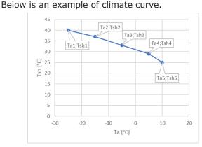
If the unit is controlled according to ambient temperature and its effect on the heating curve is enabled, the unit will change the water temperature setpoint in heating mode at fixed time intervals, based on the difference between the external air temperature measured and the relevant setpoint. The resulting difference is then subtracted from the water temperature setpoint that has been calculated according to the climate curve.
